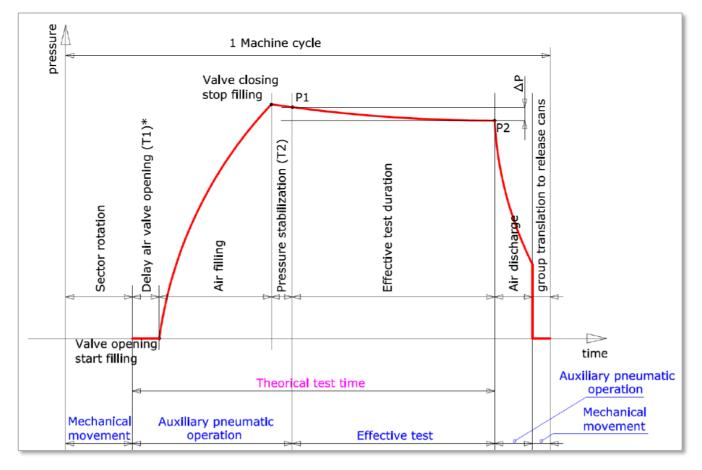
According to the values comparison and the data stored into the PLC, the machine detects the leaking tubes which will be ejected from the production flow. It means that all the tubes that compose a batch are controlled.
